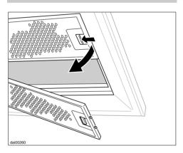
■ To remove the grease filters press the locking clips in towards the middle of the filter. Support grease filter so that it does not fall on to the cooktop.
